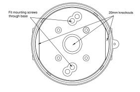
Fig 2 Mounting Beacon Base.
